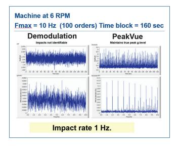
Second, PeakVue uses a fixed sample rate of 102,400 samples per second. In normal vibration data acquisition, the sample rate is calculated from the selected Fmax where the sample rate = Fmax x 2.56 to ensure that no signal aliasing effect is permitted. For normal vibration, setting a low Fmax results in a low sample rate. In PeakVue, the sample rate is fixed at 102,400 samples per second, which permits data capture and analysis of high-frequency stress waves, even for slow speed equipment.
