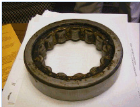
Figure 19. Photography of the defective bearing highlighting the "caked" residue of lubricant and skid of roller 5.
