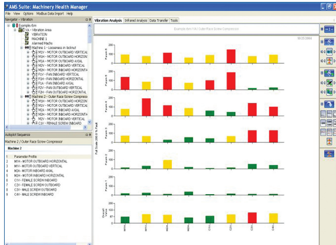
Quickly determine the status of a machine with the Parameter Status Profile.
